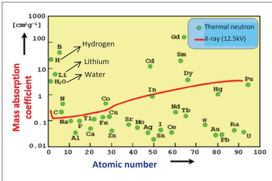
Figure 9: Absorption Coefficient of X-ray and Neutron Beam: Dependence on Atomic Number
