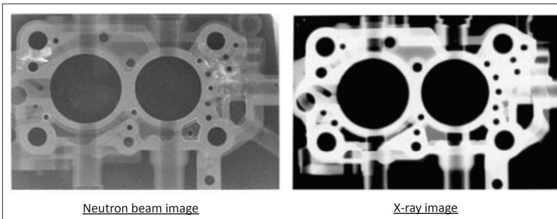
Figure 10: Transmission Image of an Engine
