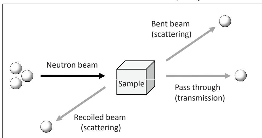
**Figure 2:** Material Analysis Using Neutron Scattering and Transmission
