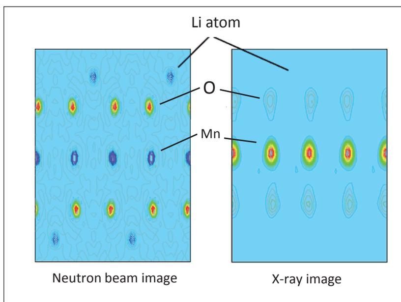
**Figure 7:** Structural Analysis of Lithium Ion Battery Cathode Material
