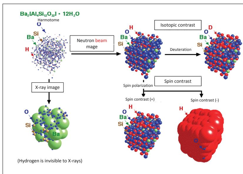
**Figure 6:** Schematic Representation of Structural Analysis Using Neutron Beam
