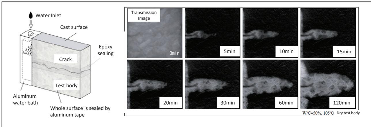
Figure 11: Infiltration of Water Through Concrete Cracks (Time Change)
