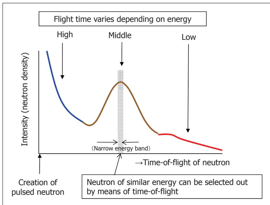
**Figure 4: Energy Selection Method for Pulsed Neutrons**
