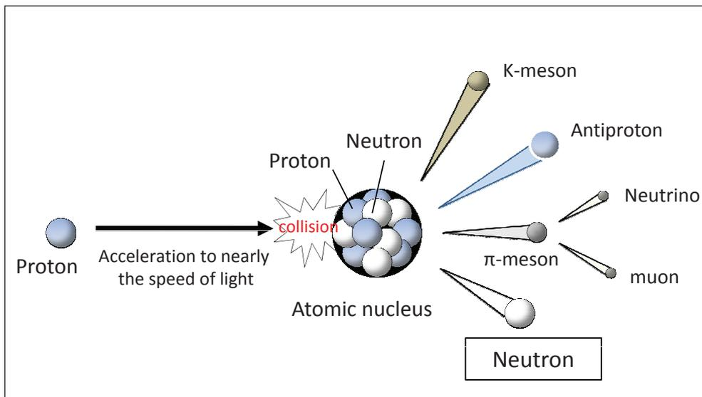
**Figure 3: Neutron Creation Using an Accelerator: Nuclear Breakdown**
