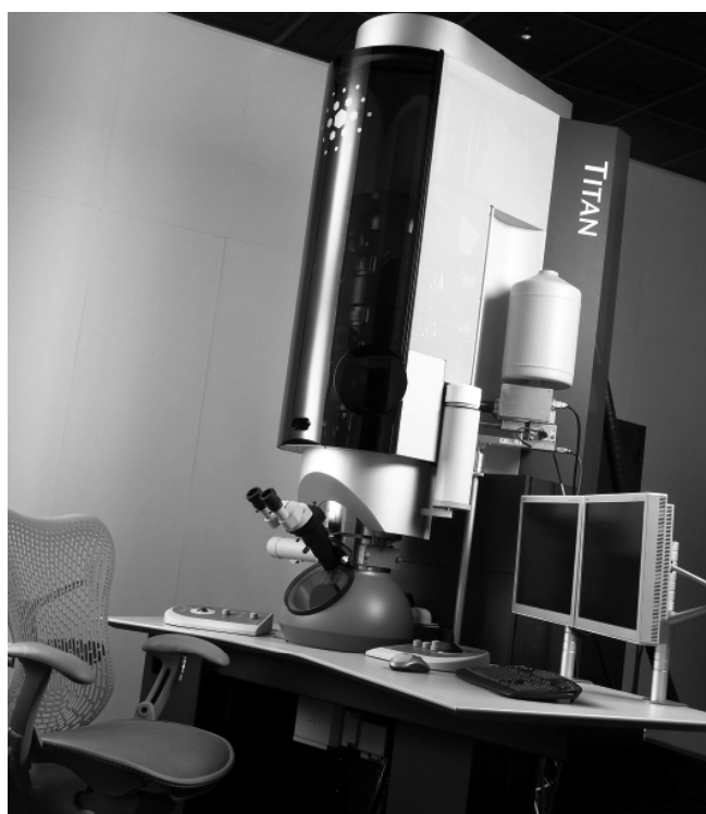
Figure 8: TITAN (acceleration voltage 300 kV): FEI's aberration-corrected electron microscope
