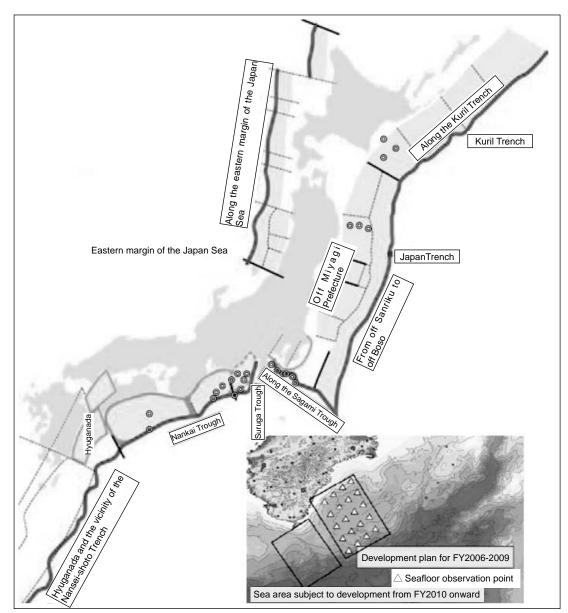
Figure 7 : Assumed Subduction-zone Earthquakes and Cabled Seafloor Seismographs ( ◎ ) Bottom right figure: the Dense Oceanfloor Network System for Earthquakes and Tsunamis being developed by JAMSTEC in Kumanonada for Nankai Trough earthquakes
