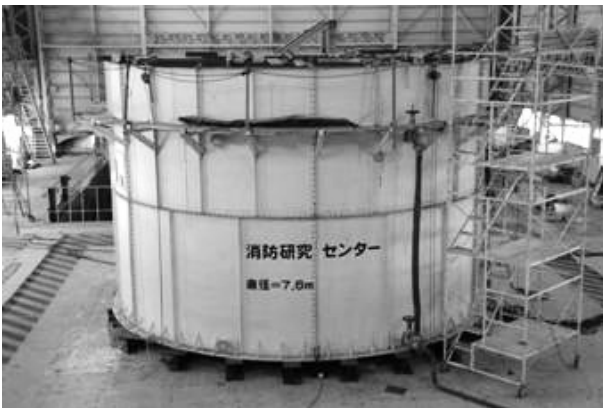
Figure 8 : Sloshing experiment using a model tank
