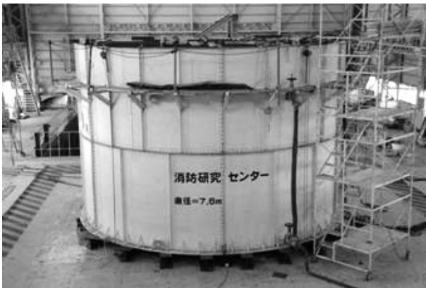
Figure 8 : Sloshing experiment using a model tank
