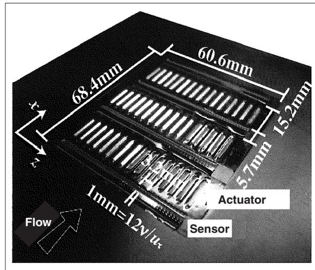
**Figure 6** : Feedback control system for wall turbulence
