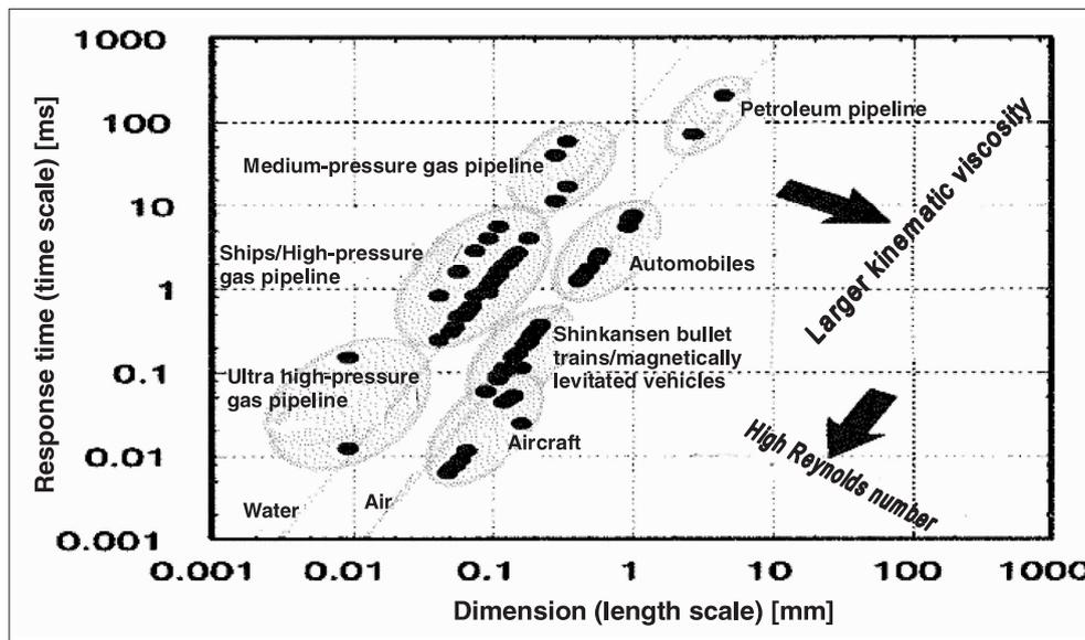
**Figure 4 :** Specifications for sensors and actuators used for longitudinal vortex control
