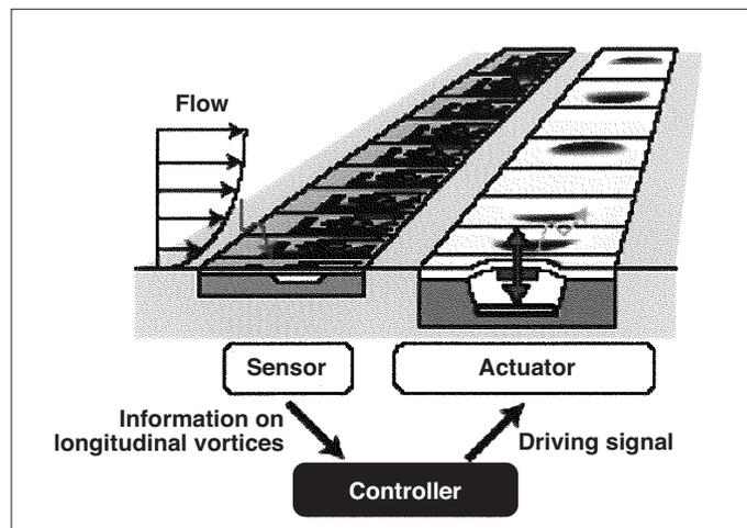
**Figure 5 :** Schematic diagram of a feedback control system for wall turbulence
