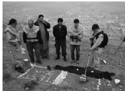
Figure 4 : Typical ALIS detection images CDS site in Afghanistan. The target is an inactive PMN-2 landmine.
