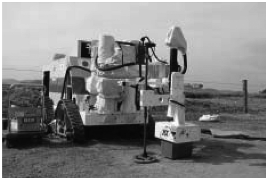
Figure 7 : A compact Mine Hunter Vehicle (Chiba University) equipped with SAR-GPR (Tohoku University)
