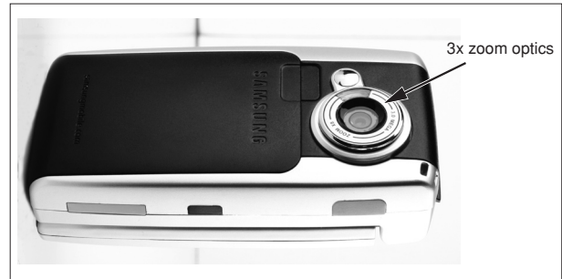
Figure 8 : Prototype of a camera-phone with conventional 3x zoom optics
