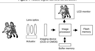
Figure 1: Basic digital camera construction
