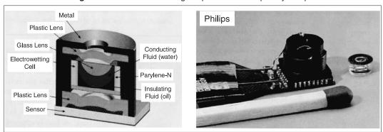
Figure 12: Tunable-focal-length liquid lens developed by Philips
