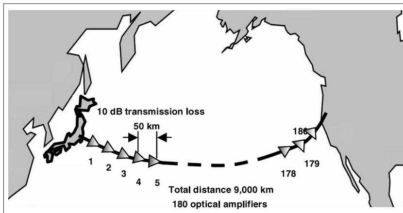
Figure 4 : Structure of the optical communications network
