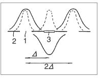
Shift phases of adjacent patterns on the mask by 180 degrees for a resolution improvement of about twice
