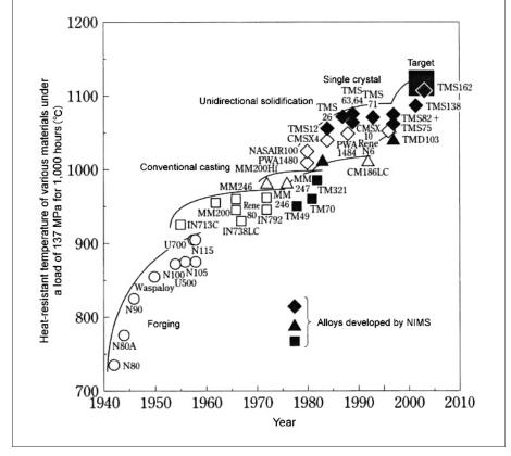
Figure 5: History of improvement in the heat-resistant temperature of nickel-base superalloys<sup>[10]</sup>
