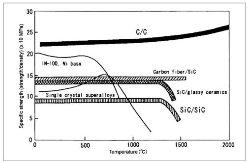
Figure 7 : High temperature strength of various composite materials<sup>[14]</sup>
