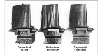
Figure 6 : Turbine rotor blades fabricated by conventional casting, unidirectional solidification, and single crystal solidification<sup>[12]</sup>
