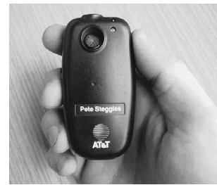
Figure 3: A Bat, a compact handheld terminal consisting of 2 buttons, 2 LEDs and a beeper
