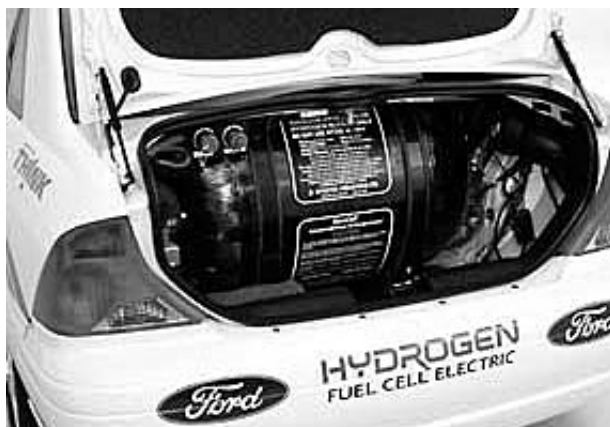
(a) 350-atm. Pressurized hydrogen tank placed in the trunk space of a passenger car.
