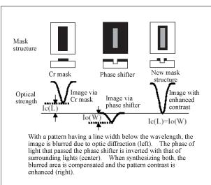
Figure 1: Contrast enhancing technology presented by Matsushita
