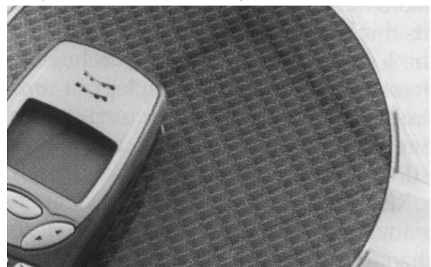
Figure 6: MEMS chips arranged on a silicon wafer [1]
