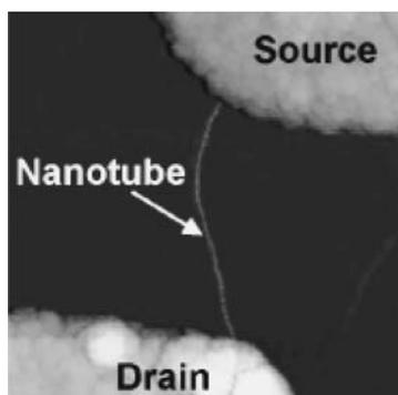
(Interval between the source and drain electrodes is 1  $\mu\text{m}$ .)
