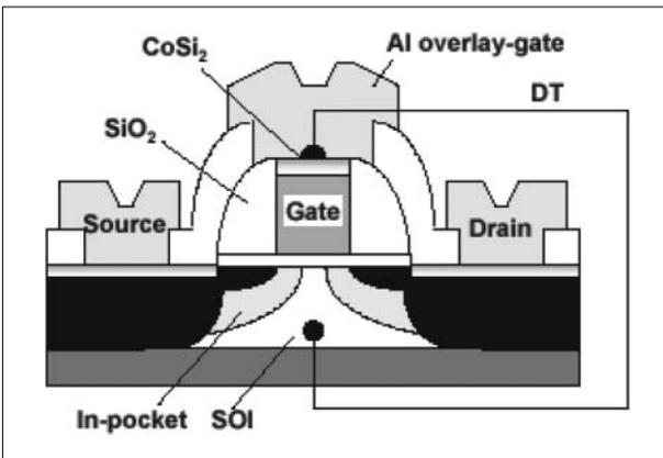
structure where the gate electrode is connected to the body.
