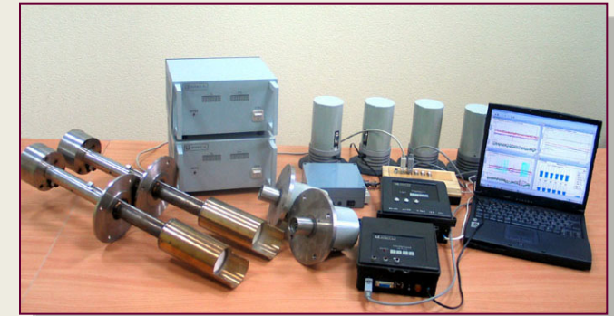
Multispectral (UV, visible, IR) sensors and gasanalyzers of the system
