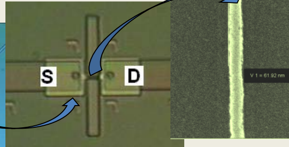
SOI-NWT source (S), drain (D), connected with 50 nm nanowire
