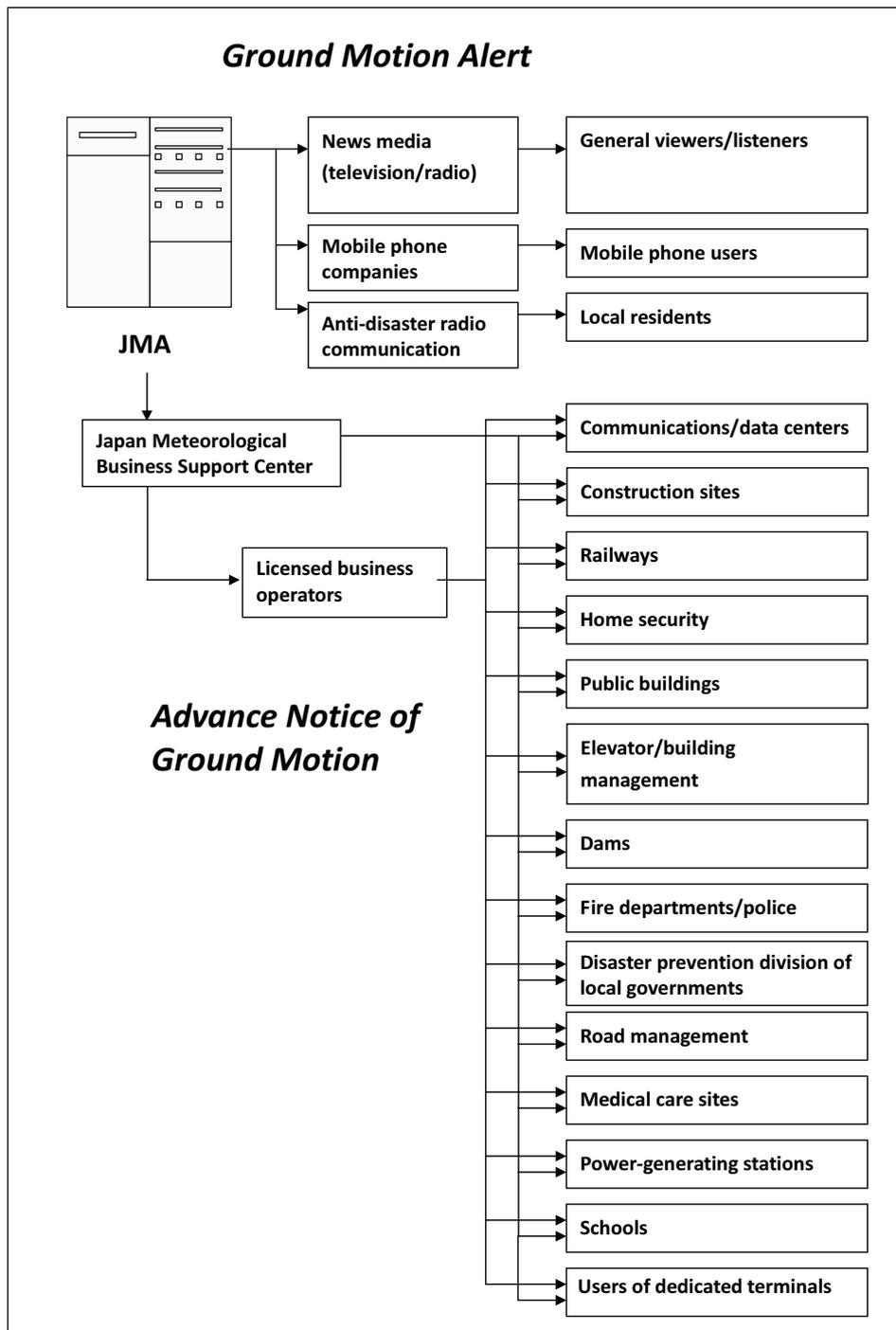
**Figure 3 :** Transmission Patterns of Earthquake Early Warnings
