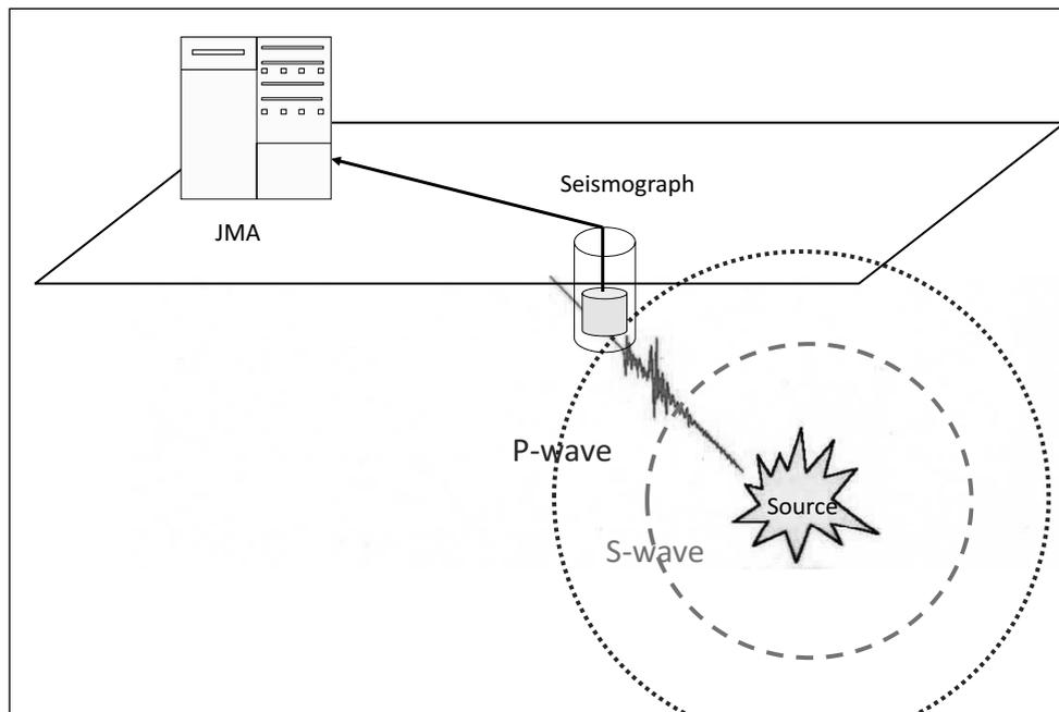
**Figure 1 :** Principle of the Earthquake Early Warning
