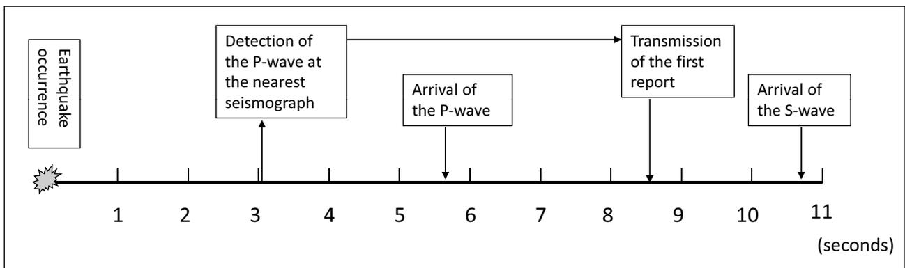
**Figure 2 :** Time Chart of the Seismic Wave and Transmission of an Earthquake Early Warning
