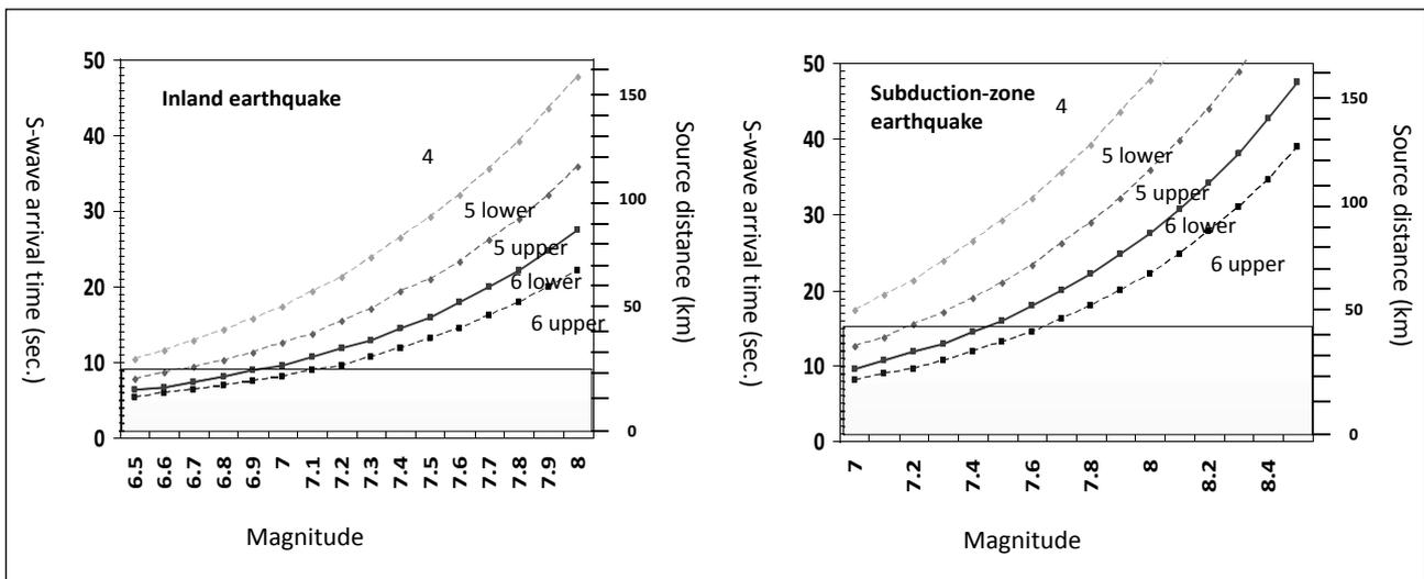
**Figure 4 :** S-wave Arrival Time by Seismic Intensity
