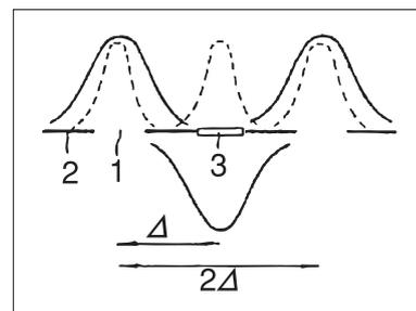
Shift phases of adjacent patterns on the mask by 180 degrees for a resolution improvement of about twice
