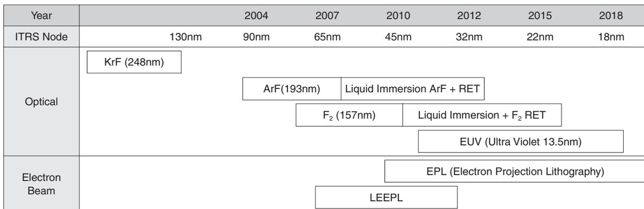
called ITRS (International Technology Roadmap for Semiconductor) and is defined by major electronics companies in the world including Intel Corporation in U.S.A. At first, the minimum line width was in the order of microns, and this continuously decreased over time, and now a 90-nm node will be in production with the size of a DRAM with this line width corresponding to 4 Giga bits. The target for 15 years from now is set to an astonishing 18-nm line width for 128-Giga-bit capacity.
