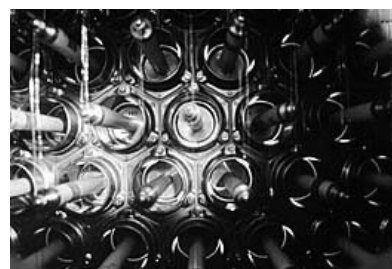
Figure 4: Interior of a typical ozonizer
